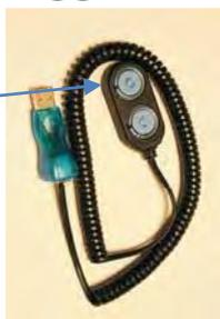
The logger is the small “watch battery” looking device that may be on a plastic holder. The logger will “click” into place. The details tab should now appear with the following options available:
