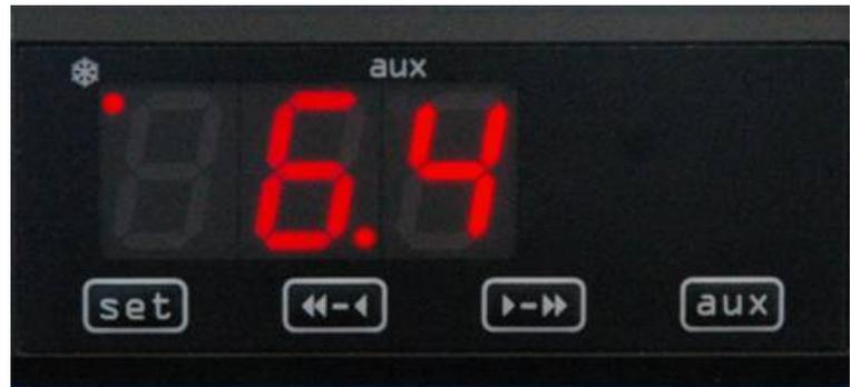
The current set point for the fridge can be checked by depressing and holding down the SET button. This will typically show 3.0.
