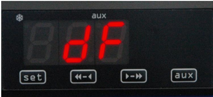
By holding “◀◀ - ◀” and “▶ - ▶▶” buttons together this forces the fridge into defrost mode for the programmed time and will then continue its normal operation.
