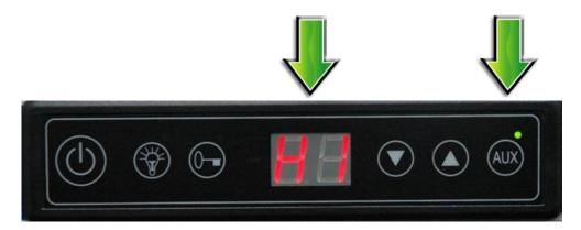
If the high alarm is going off it may be from the door being open or a power cut if one has occurred. If it starts beeping again after you have turned the alarm off, please get in contact with us.
