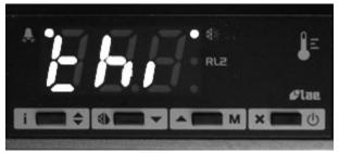
The controller alarm is typically set to go off if the fridge is below 2° or above 8° for more than 10 minutes. The display will read "HI" or "LO" and the alarm will continue to sound until any button has been pressed. If the "HI" alarm is going off it may be from the door being left open or a power cut if one has occurred.
