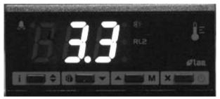
The current set point for the fridge can be checked by pressing and holding the "I" button. This set point is showing 3.3°C. This will typically show around 3.0°C. This can be adjusted by pressing and holding the "I" button and using the " $\nabla$ " and " $\Delta$ " buttons to suit.
