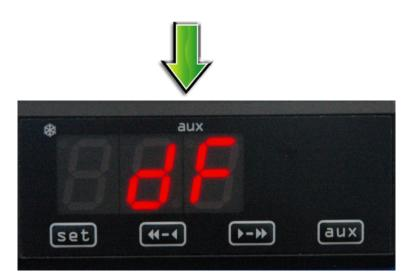
By holding "◀◀ - ◀ "and "▶ - ▶▶" buttons together this forces the fridge into defrost mode for the programmed time and will then continue its normal operation.
