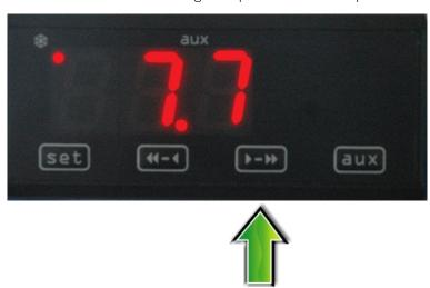
To reset the high temperature in memory, hold the temperature button and press "set" at the same time.
