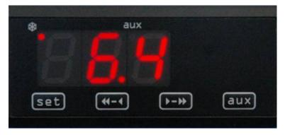
The current set point for the fridge can be checked by depressing and holding down the SET button. This will typically show 3.0.
