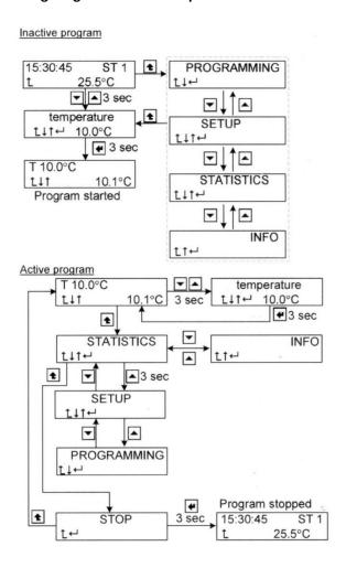
To stop the programme, press the exit **L** button twice. You will see STOP on the display. Press and hold the enter **L** button for at least 3 seconds.
