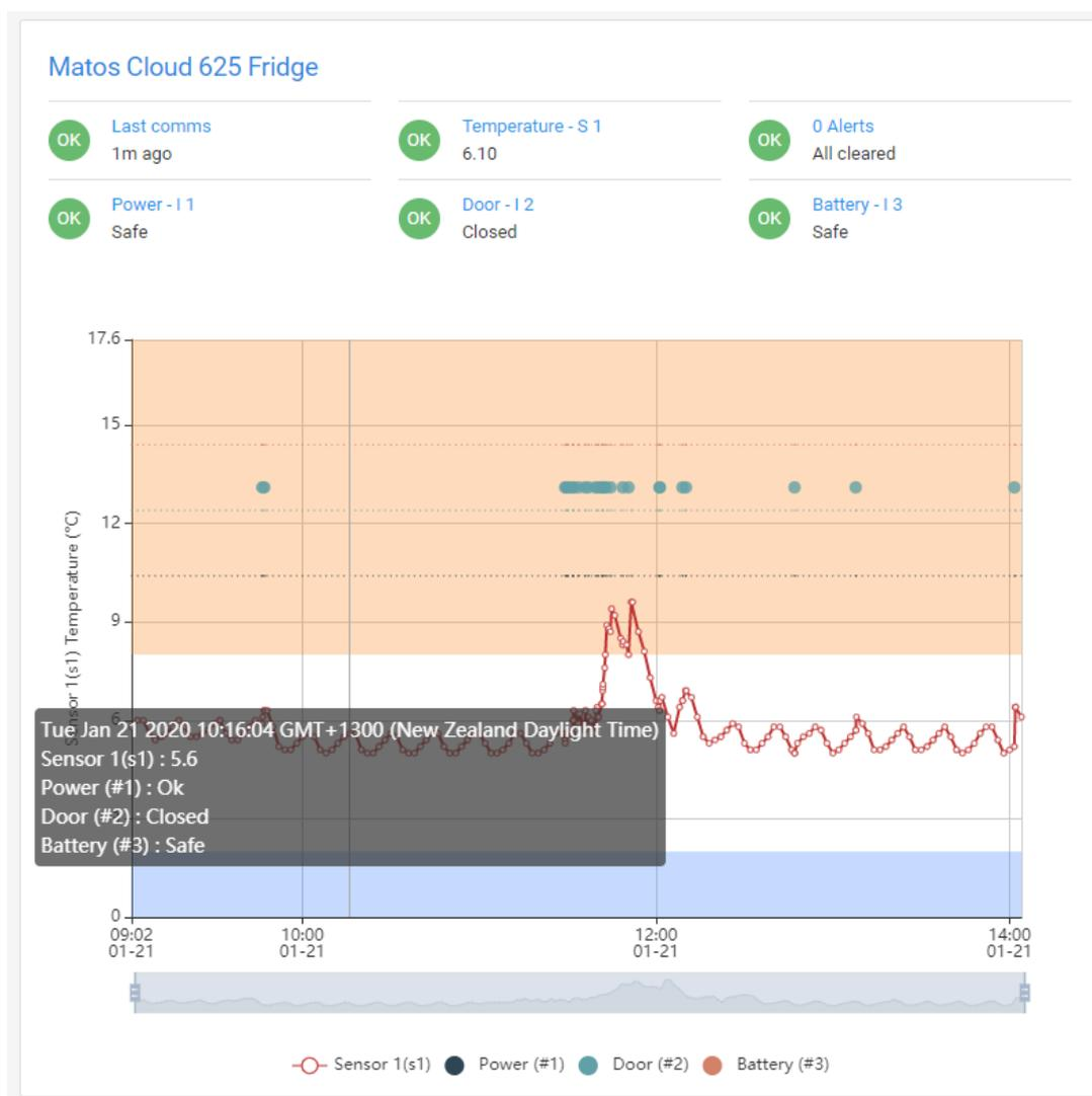
To the right of the graph, there is also a table showing the current status as applicable to the current asset. E.g. if there is a door input assigned, the status of this will be displayed here. All assets will display at least the last communication time, Sensor 1 value, and alert status.
