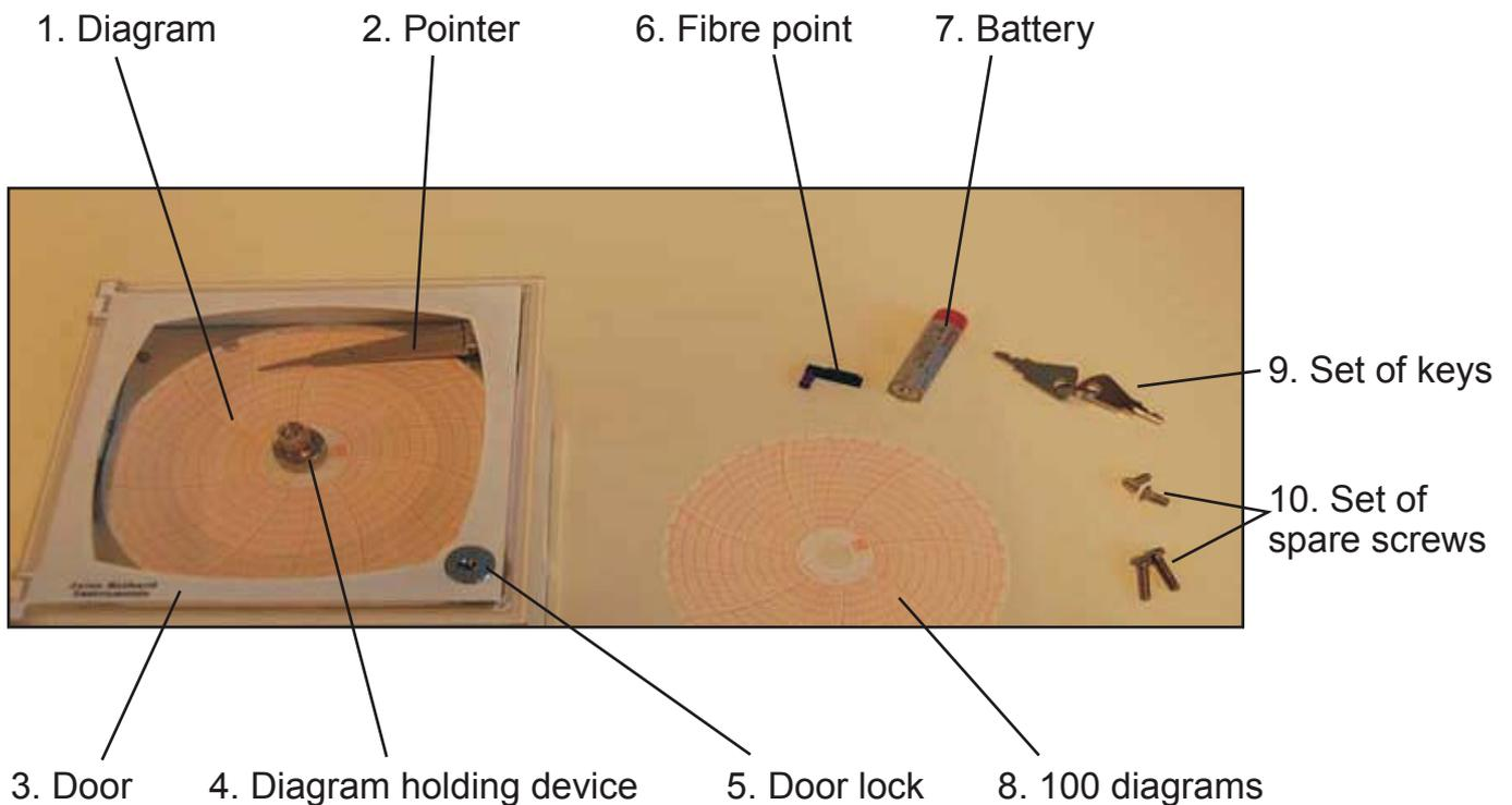
The Chart Recorder is device intended to monitor the temperature.
