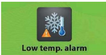
The **Low temperature alarm** indicate, that the temperature inside the unit is lower than permitted from setting of the unit.
