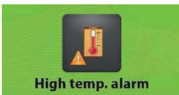
The **High temperature alarm** indicate, that the temperature inside the unit is higher than permitted from setting of the unit.
