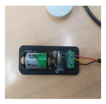
3. Take out the old battery (take note of which way the battery is to be inserted - Positive points to the wires). Now fit the NEW Battery.
