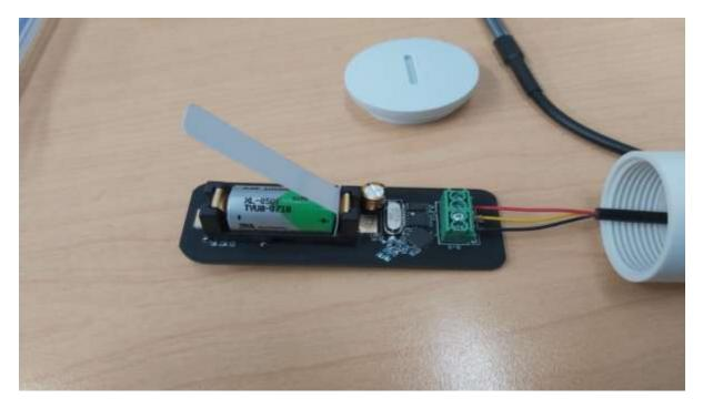
3. Pull the white plastic battery tab out. It may be easier to remove the battery completely and then replace. Take note of which way the battery is to be inserted (Positive points to the wires).
