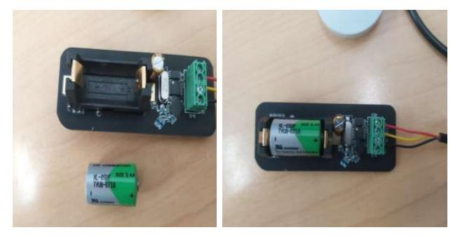
4. Slide the circuit board back into the white tube and replace / tighten both end caps. <u>The sensor</u> is now ready to go.
