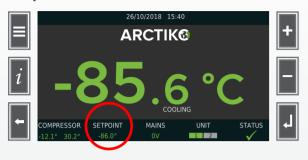
Press the UP to increase the temperature or the DOWN to decrease the temperature. Once the temperature has been set press ENTER to save the new value and exit.
