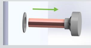
2. Rinse the valve on the exterior side with cold tap water for 2 to 5 minutes or until all ice inside the valve is removed. Make sure the vacuum valve is completely dry before inserting it into the tube and be aware that it is inserted correctly (push it firmly until it clicks in).
